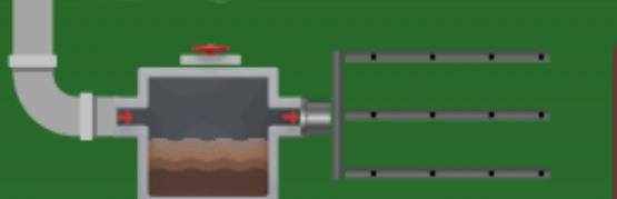
**SEPTIC SYSTEM** - treats wastewater on-site. Solids are filtered in the tank and effluent is dispersed into the ground for natural filtration of bacteria.
